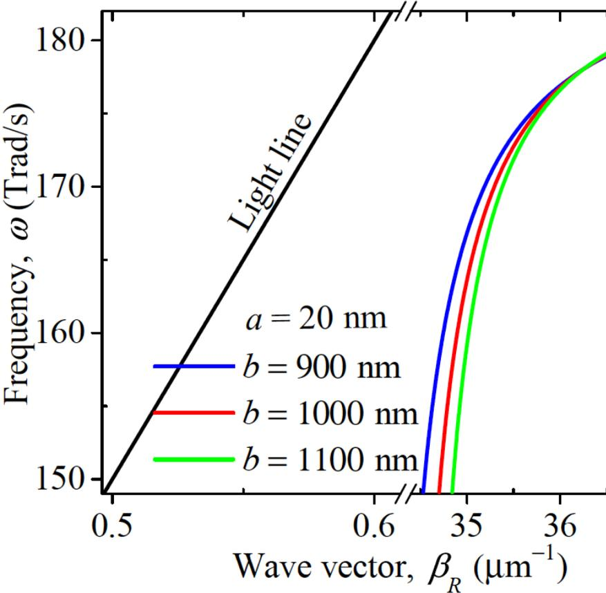
A size change of 200 nm does not affect significantly neither the dispersion relation nor the propagation length.
