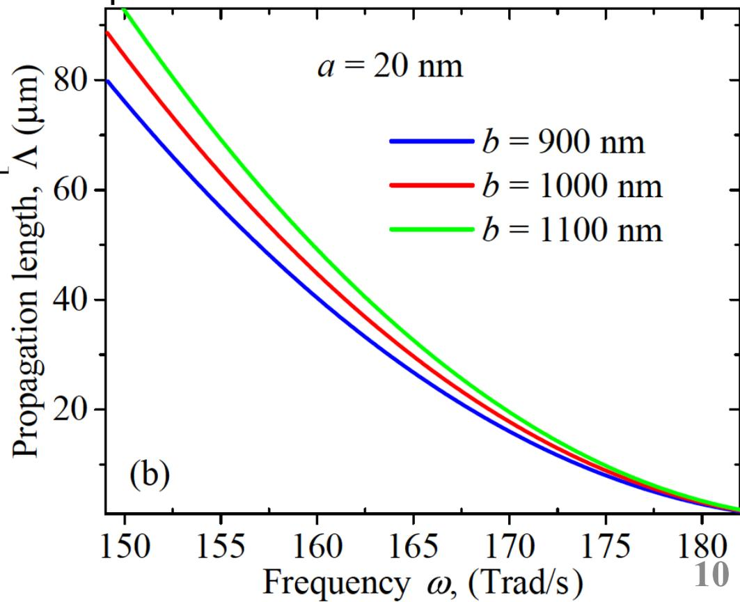
For  $b \gg a$ , the SPhP energy is not significantly modified by the nanoparticle size dispersion.
