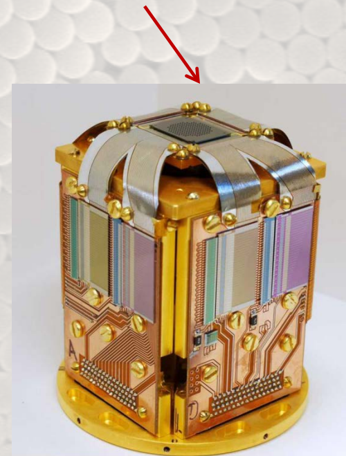
0.1 K TES X-ray detector array and SQUID readout, NIST+JYU
